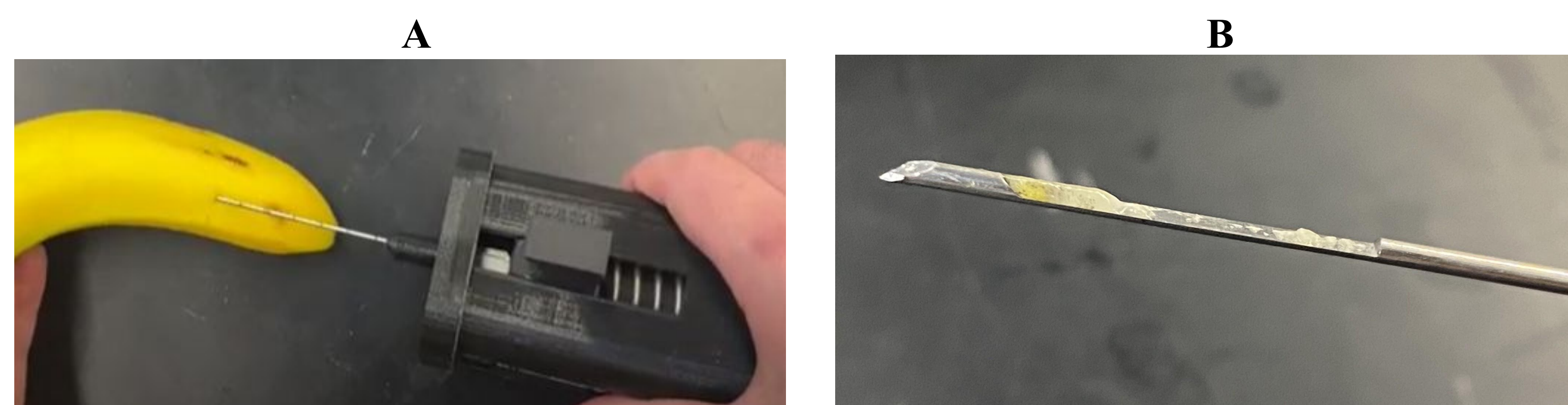
Figure 8. (A) Image of prototype being inserted into a banana. (B) Sample collected in needle well after firing device.
