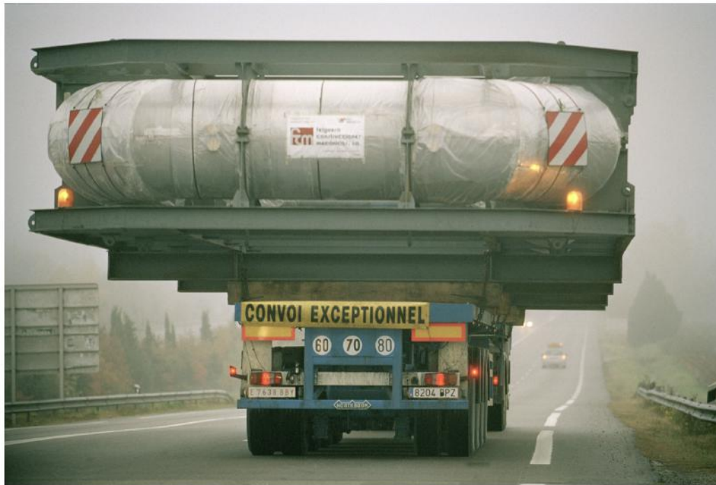
Figure 6: Road transport of a structure for the ATLAS air toroids. Photo reproduced from Ref. [181].
