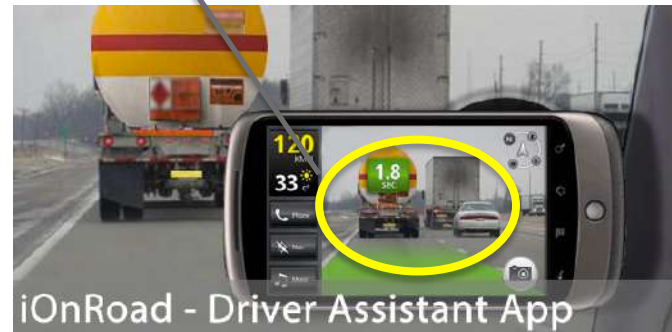
iOnRoad - Driver Assistant App Smart phone Example: Forward Collision Warning
